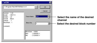
7. Click the [OK] button to load the waveform data to the channel that was selected in step 2. Only one block of a channel can be loaded with one operation.
