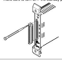
When connecting the output signal wire to the clamp type terminal, loosen the screw holding down the clamp, insert the output signal wire into the opening, and then tighten the screw.
